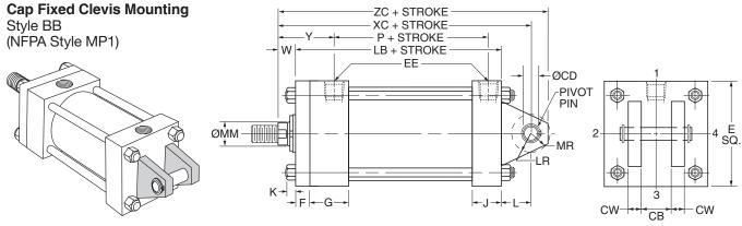
Table 1 – Dimensional and Mounting DataNote: Tie rod nuts are supplied on both ends, as shown, on 1.00, 4.00 and<br/>5.00 bores. Tie rods are threaded into the cap on all other bore sizes.
