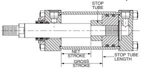
Use the following steps to determine the need for stop tube and, if required, how long it should be.
