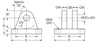
Note: Cast ductile iron clevis brackets must not be welded in place.
