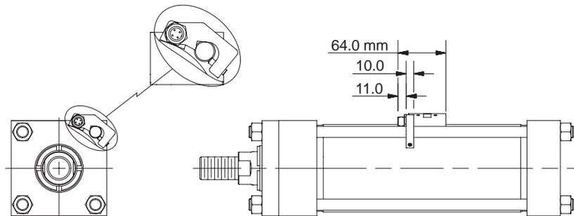
ALS Switches allow a .38 - .50 inch stroke-to-piston travel for end-of-stroke mounting locations.
