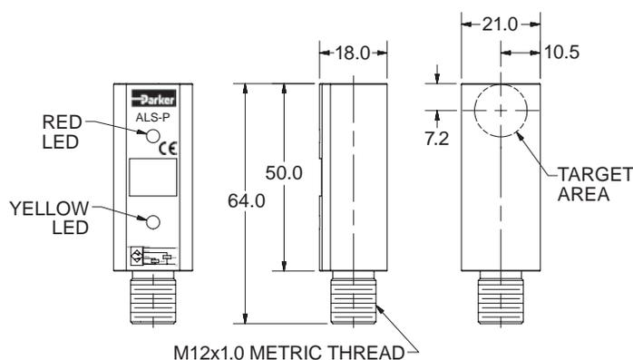
ALS Switch output states may be influenced by an external magnetic field. Care must be taken to avoid external magnetic field exposure.
