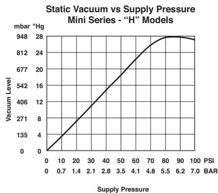
Notes: Standard operating pressure for IMI Norgren pumps is 80 PSI [5.5 bar]. Pumps can be factory modified to run at other operating pressures i.e. 60 PSI [4.1 bar] etc. The values shown in the performance chart will remain the same for all operating pressures.
