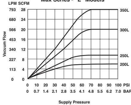
**Static Vacuum vs Supply Pressure
