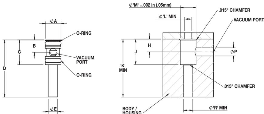
Min Series Cartridge dimensions are the same for nylon and brass
