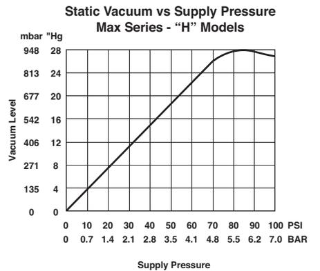
Notes: Standard operating pressure for IMI Norgren pumps is 80 PSI [5.5 bar]. Pumps can be factory modified to run at other operating pressures i.e. 60 PSI [4.1 bar] etc. The values shown in the performance chart will remain the same for all operating pressures.
