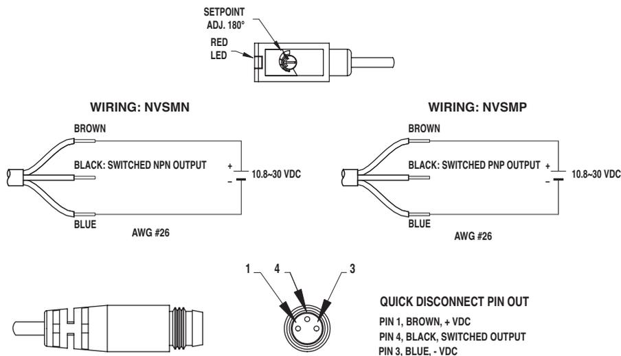
● NVSM (N or P)-QD-6 Electronic Vacuum Switch Specifications:
