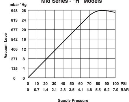
Notes: Standard operating pressure for IMI Norgren pumps is 80 PSI [5.5 bar]. Pumps can be factory modified to run at other operating pressures i.e. 60 PSI [4.1 bar] etc. The values shown in the performance chart will remain the same for all operating pressures.
