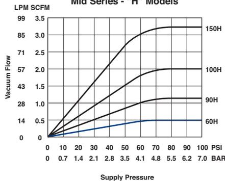
Static Vacuum vs Supply Pressure
