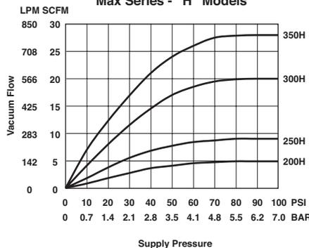
**Static Vacuum vs Supply Pressure
