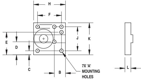
Bracket accepts: NVP00, NVPOX, NVP10 & NVP1X Series pumps and NMB18-25 manifold block.
