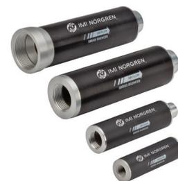
The NST Series Silencers are designed with a straight through flow path that eliminates clogging by allowing the contaminants to pass directly through the silencer. Each silencer is tuned in proportion to its exhaust flow to minimize noise.
