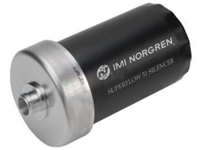
The NFA-51 Series silencers offer remarkable noise reduction for high volume exhaust applications without causing back pressure. These silencers are ideal for quieting large air valves that must exhaust quickly to maintain high cycle rates. IMI Norgren uses the FNA-51 silencers on all high flow venturi vacuum pumps where even a small amount of back pressure would decrease performance.
