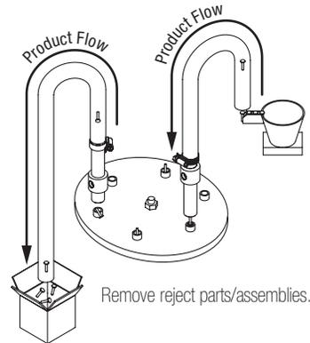
Load parts for assembly from a vibratory bowl feeder.
