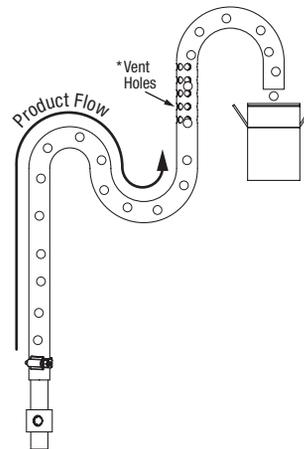
**Design Tip:** To prevent damage or to match the assembly speed, decrease the transfer speed by introducing a vertical bend into the tube, allowing gravity to work against the direction of travel.
