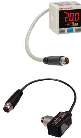
IMI Norgren's ultra-mini electronic vacuum sensors provide continuous voltage output (1-5v) proportional to the system vacuum level. Connected to a feedback interface such as a digital display or PLC, the NVTMV-QD-6 is a cost effective, reliable sensor that maintains application consistency. Sensors can be mounted directly to IMI Norgren's Modular NVP Series pumps.
