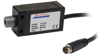
IMI Norgren's miniature electronic vacuum switches monitor vacuum levels in systems and provide a switched output. The NVXX Series has both adjustable set-point and hysteresis and an LED indicator and can be mounted directly onto a wide variety of IMI Norgren pumps. Complete with M8, 3-pin connector.
