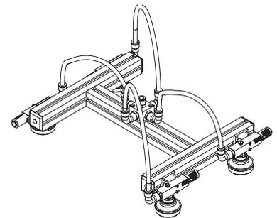
Increase safety, reliability and speed by using one pump and one cup at each location. Should one cup fail the others will maintain their grip.
