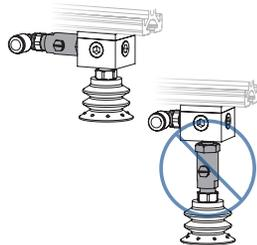
Vacuum check valves are not designed to directly support load bearing forces of any kind.
