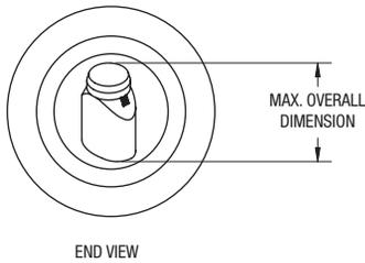
To size a NDF pump for transferring individual items, choose the pump with an inside diameter just slightly larger than the largest dimension of the object.
