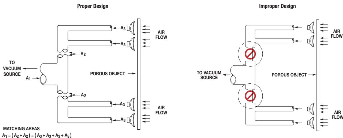
Plumbing a vacuum system is very similar to a municipal water distribution system where the lines closest to the pump are the largest and get smaller as they get to your house (vacuum cup/vessel). The area of each branch of tubing should match that of the next branch and the main trunk line should be sized to handle the maximum flow.
