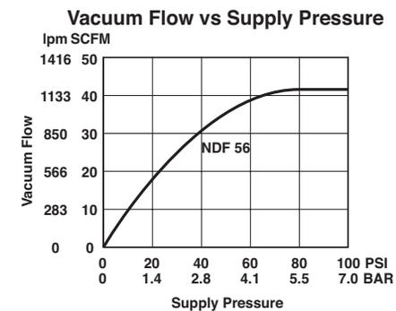
**Operating Note:** Above 40 PSI [2.7 bar], the increased energy consumed through rising air consumption is converted into increased vacuum level while vacuum flow stays constant. It is the vacuum flow that provides the motive force for the materials to be transferred. Higher vacuum levels are useful when lifting high molecular weight bulk materials and heavy individual objects long distances vertically.
